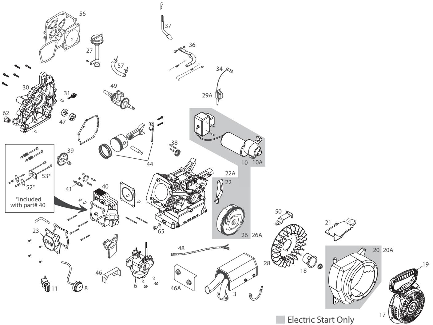
**REPAIR PARTS SNOW THROWER - - MODEL NUMBER PR621 (96182000301)**
