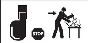
Always stop unit and disconnect spark plug before cleaning or servicing.
